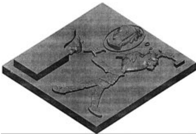
Fig. 11. Shaded image of the sculptor converted to an STL file enclosed by a rectangular box.
