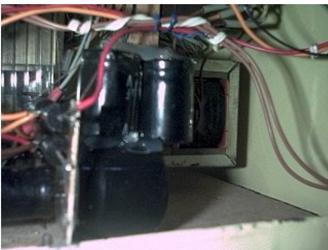
Capacitor bank (4 caps. 220uF x 200V).
