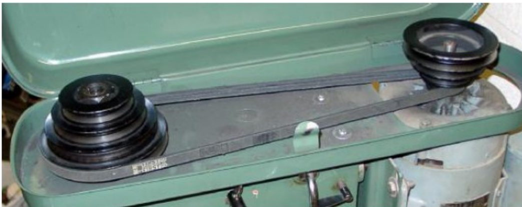
Figure 5.15 - Pulley spindle drive
