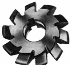
FIGURE 15—A 14-1/2° HSS involute gear cutter
