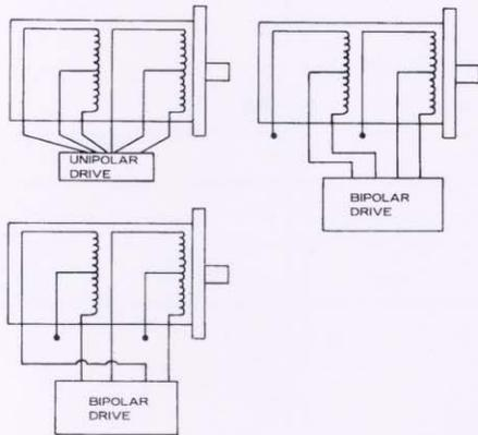
Can be driven from unipolar or bipolar drives.
