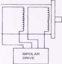
Can only be driven from a bipolar drive. Bipolar drives require 4 motor wires and energise the 2 phases sequentially with alternate polarity.
