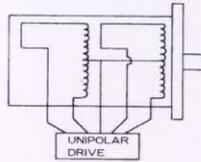
Can only be driven from a unipolar drive. Unipolar drives require 5 or 6 lead wires and each of the 4 phases are energised in sequence with no change in polarity.
