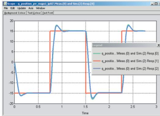
Figure 1: PV Controller: Actual and Theoretical Position Responses to a Square Wave Setpoint
