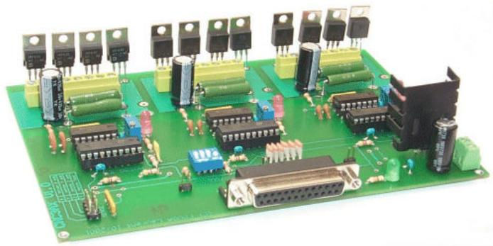
3 axis PC parallel port stepper motor control board
