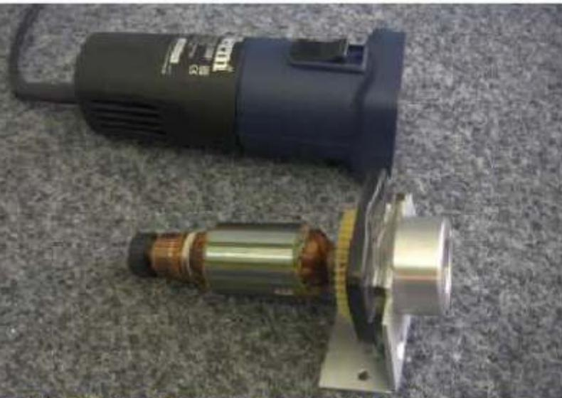
Using Loctite 330 aswell screws for assembly
