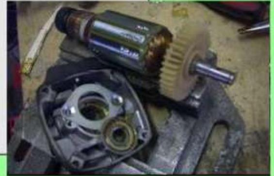
Then using a file creating a flat surface 90 degrees to the shaft
