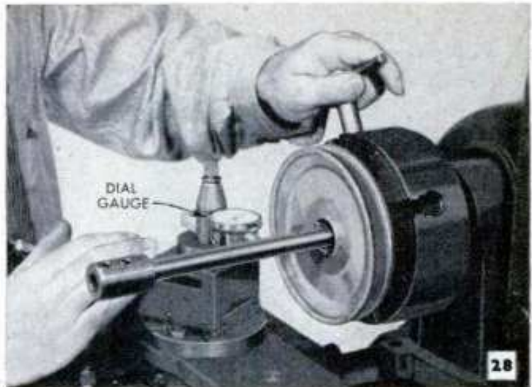
ACCURATE CENTERING IS NEEDED ON REBORING JOBS
