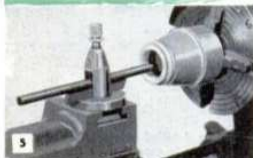
DIRECT MOUNTING IN TOOL POST
