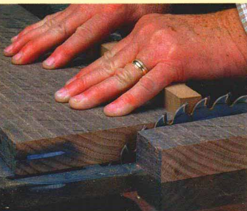
Cutting a nail. Not only does this damage a blade, but it can also send a very hot piece of metal into your saw cabinet.
