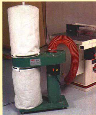
Sparks in the bag. Metal sucked into the dust collector's fan blade may cause a spark and ignite sawdust in the filter bag.
