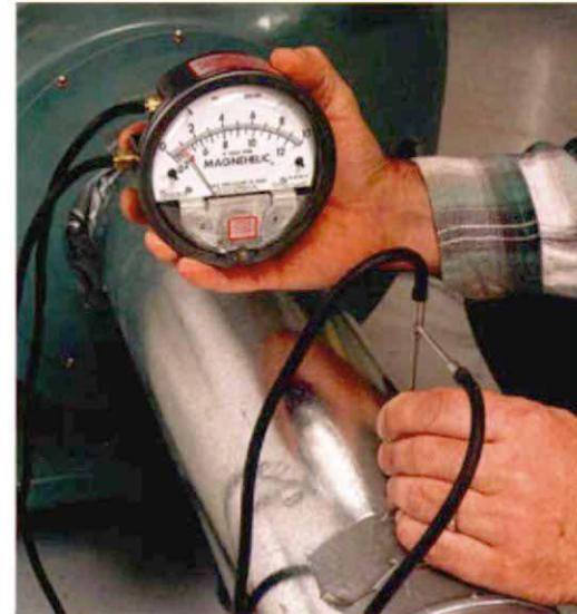
**Measurements were taken with a dial-gauge manometer (a pressure gauge) and pitot tube. The chart at right compares the performance of a few dust collectors when using hose, PVC pipe and metal duct.**
