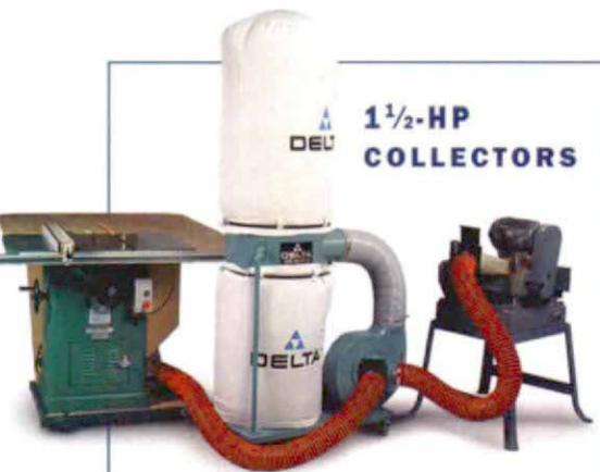
**Although collectors in this power category may occasionally be used with two tools simultaneously, for best performance, use blast gates and run one tool at a time.**
