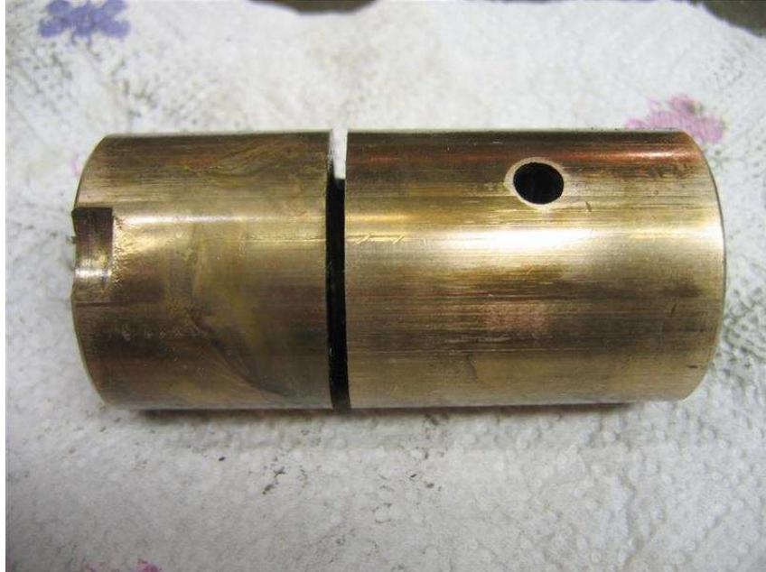
Line up the keyway in the nuts and slide it into its casting in the saddle until the distal end of the nut bottoms in its hole. Screw the large headed adjusting screw back in its hole, and tighten it until you can't easily turn the feed screw with your hand. Temporarily reassemble the cross feed bearing casting and handle onto the feed screw and check how much backlash there is in the screw. The two ends of the feed screw are least worn,
