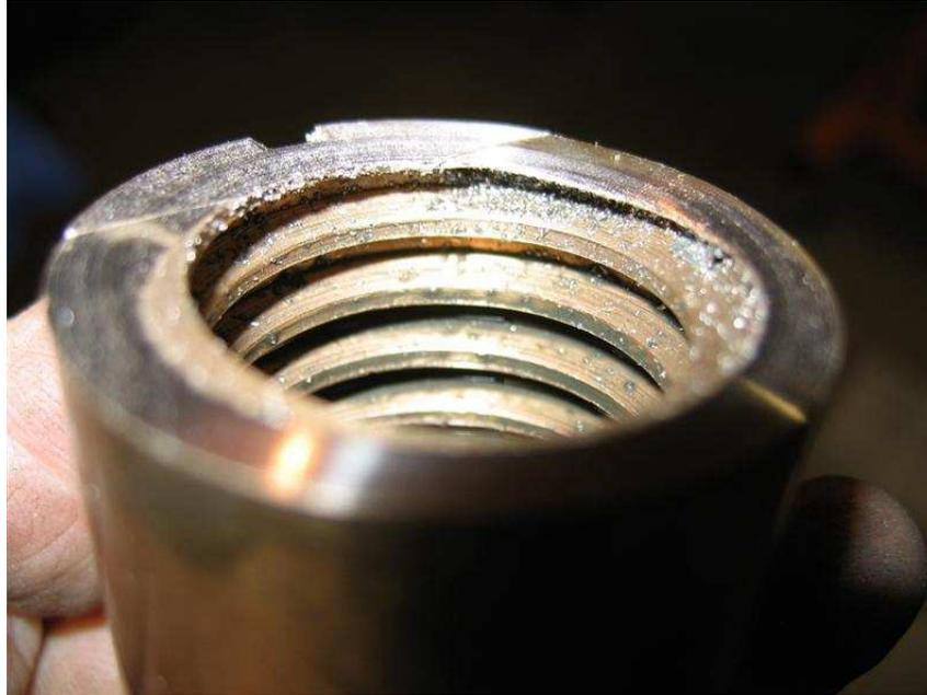
Take the time now to clean out the threads and the outside of the nuts with solvent. Clean out the holes in the casting where the nuts go. When clean, they are a push fit in the casting and the nuts can slide back and forth a little with hand pressure.
